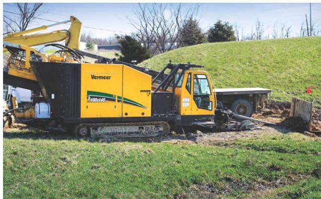
Figure 3. On shorter bores ranging between 400 - 600 ft (121.9 - 182.9 m), the crew used the Vermeer D100x120 HDD. For longer bores ranging from 1000 - 1700 ft (304.8 - 518.2 m), the Vermeer D300x500 HDD was used.
